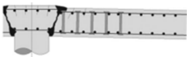
Failure closed to column by crushing of concrete
