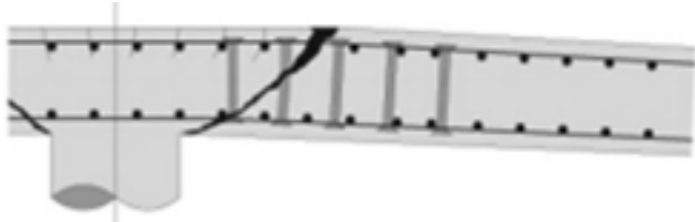
Failure within shear-reinforced area
