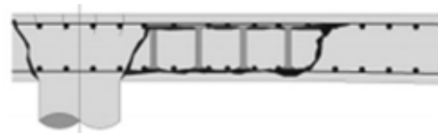
Delamination of concrete core
